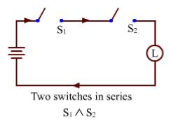
The series connection corresponds to  $S_1$  and  $S_2$ . This can be written in the logic notation as  $S_1 \land S_2 S_1 \land S_2$ .
