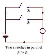
The parallel connection corresponds to  $S_1$  or  $S_2$ . This can be written in the logic notation as  $S_1 \ V \ S_2 S1 \ V S2$  .
